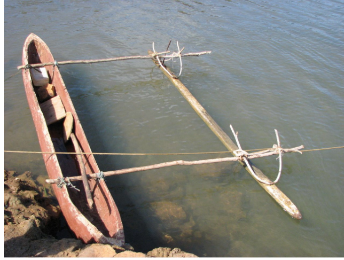
Figure 1.5: Tongan dugout with outrigger. Two booms and indirect U-shaped stanchions connect main hull to outrigger float. Low freeboard (distance between waterline and gunwale) and lack of washstrakes (added planks along sides to keep the sea out) make this canoe more vulnerable to swamping compared to that in Figure 3. Photo by A.V. Bell.
